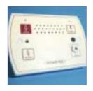
L752 audio call point – the L752 is a versatile audio call point used on every individual audio call location on the system. It features 7 levels of call, hands free two-way intercom, integral infra red receiver, audio page facility, reassurance LED and 'call follower' sounder. It will also accept a host of triggering devices including pear leads, air switches, pressure mats etc. The unit may be flush or surface-mounted using the Intercall BB1 Backbox.
